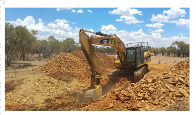
FIGURE: Excavation of bulk phosphate rock sample for crusher test work at Ardmore.
