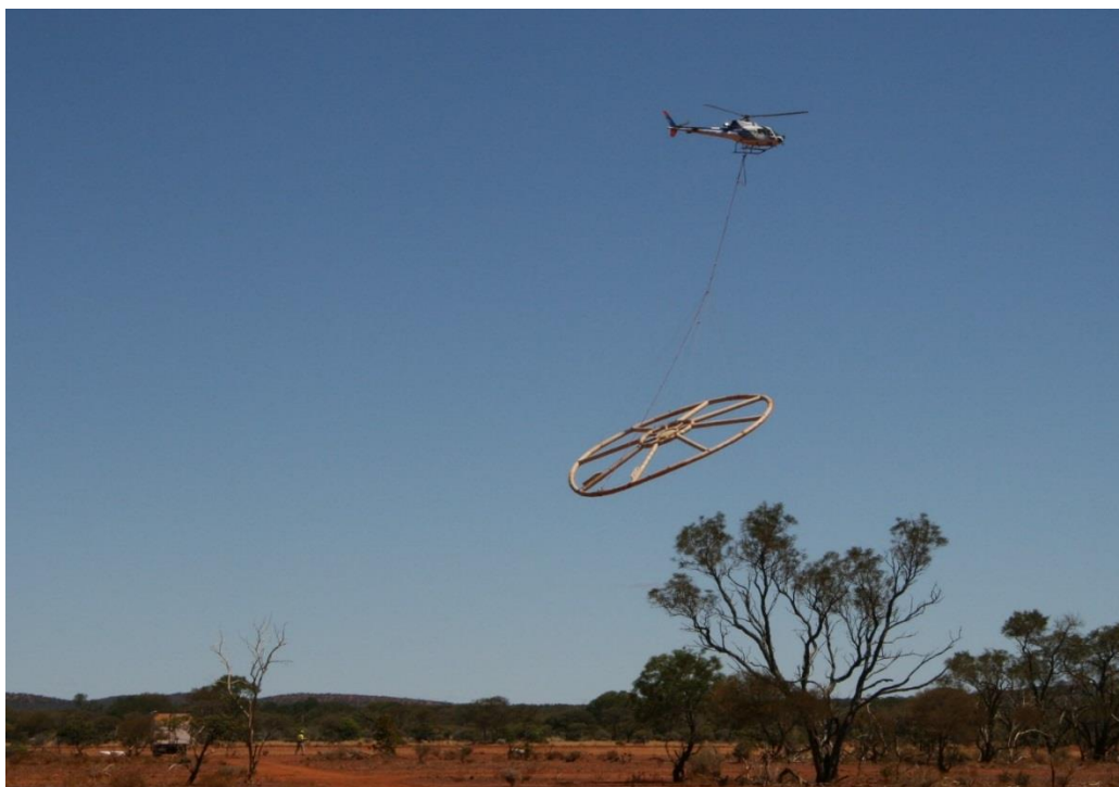
Figure 2: Helicopter-borne Electromagnetic (EM) survey underway at Woodlands
