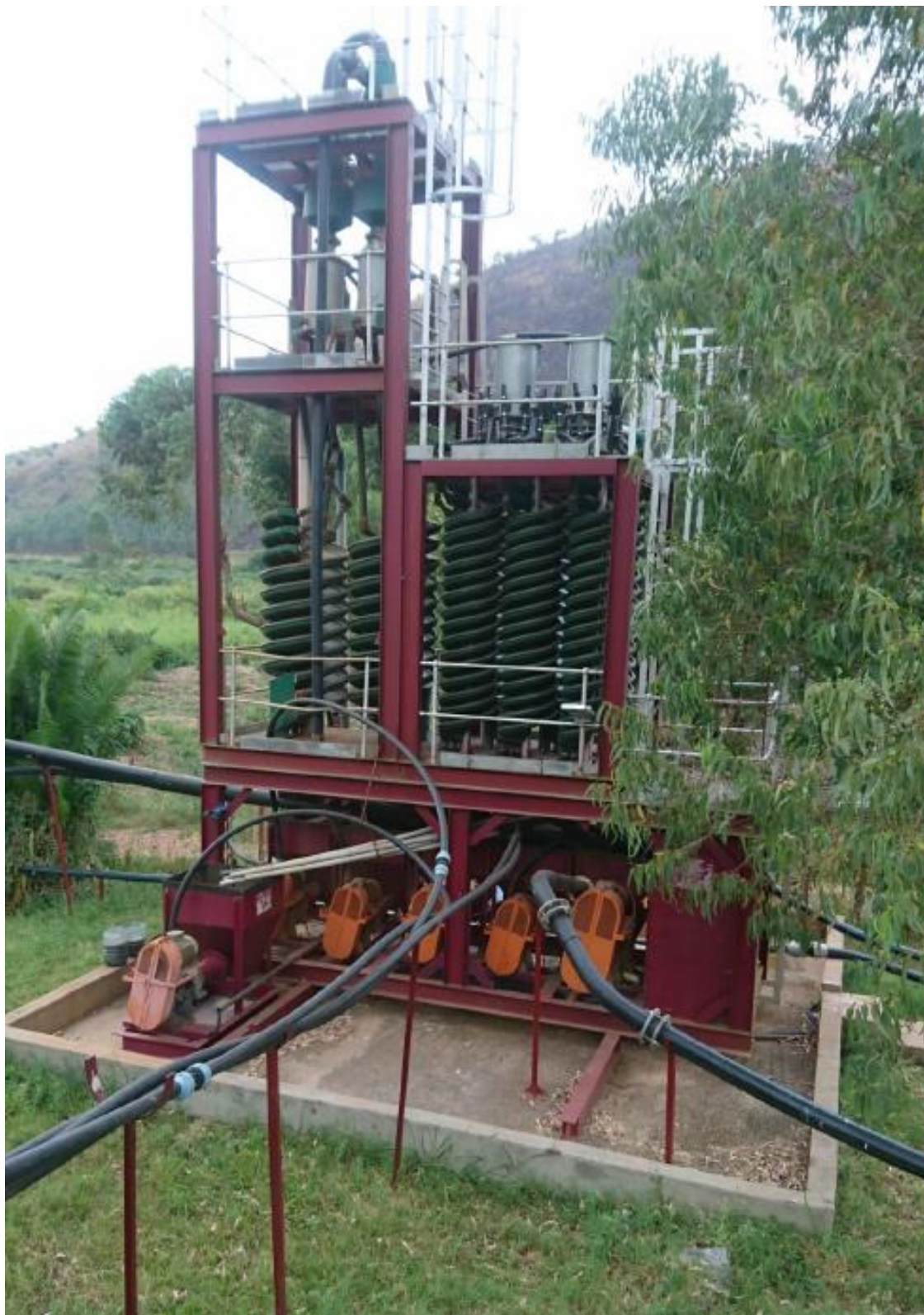
Gravity spirals used to separate the heavy tin minerals (cassiterite)
