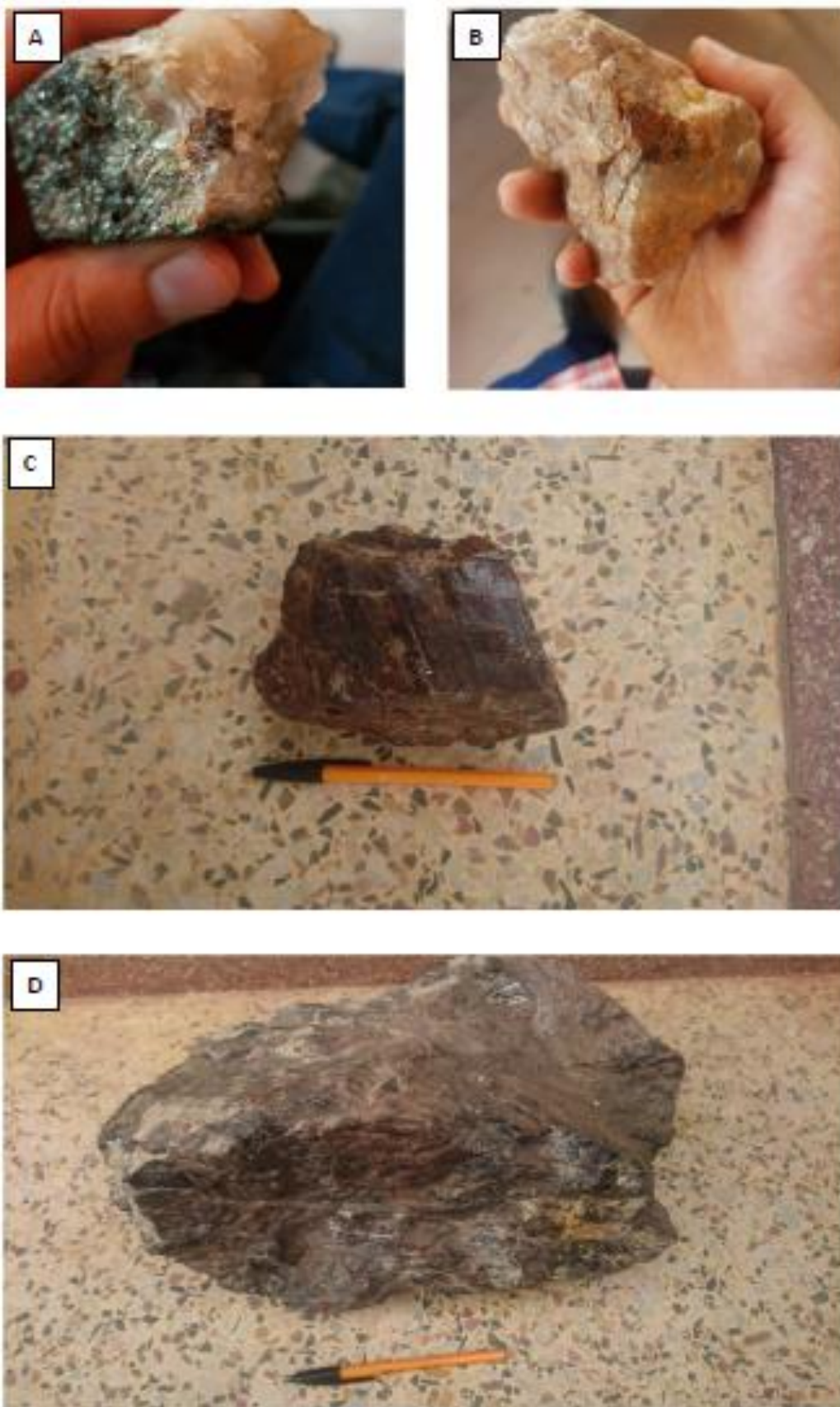
Image A and B - Cassiterite samples associated with muscovite, tourmaline and quartz veining; Image C - Cassiterite specimen approximately 15cm long; Image D – Cassiterite specimen approximately 40cm long and weighing 50kg
