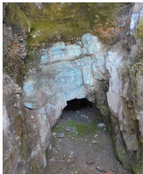
Figures 2 and 3: Azurite copper oxide mineralisation in subvertical brecciated quartz (left) and the shallow dipping copper clay horizon(right). Fields of view of the brecciated quartz vein with azurite outcrop on right is approximately 5 metres and the adit in sub-horizontal copper clay approximately 3 metres.
