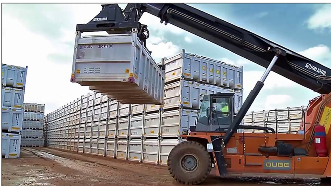
Figure 11a. Movement and stacking of Qube Rotabox containers at the berth
