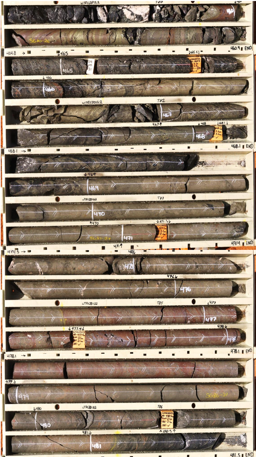
Figure 1 - WTRCDD122 Highlights: Massive/Semi-massive pyrite-sphalerite-galena-chalcopyrite
