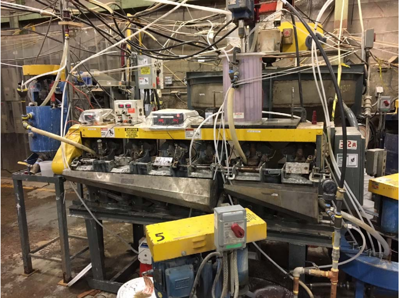
Figure 3: Spodumene rougher flotation
