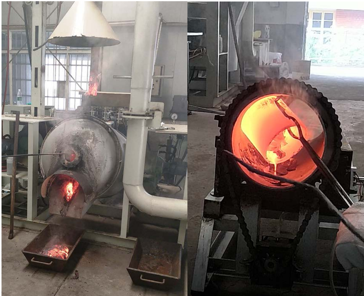
CAPTION: Oxley electric arc furnace trial (left), and rotary cooler trial (right).
