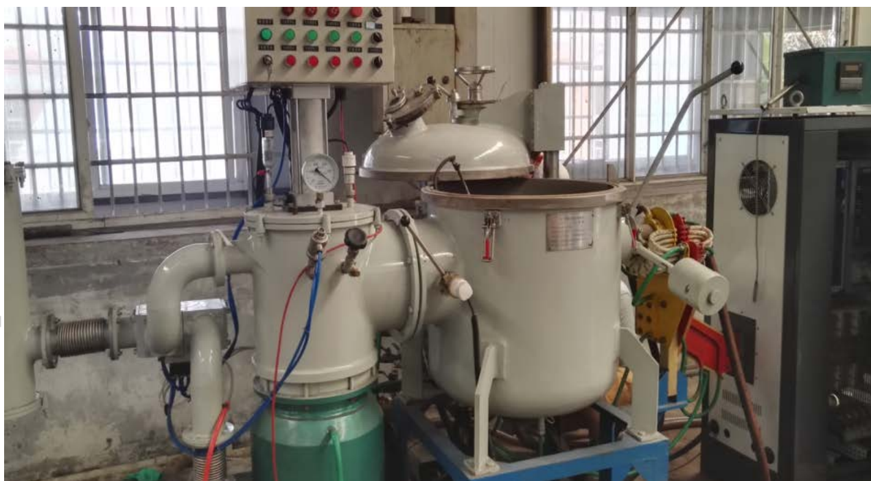
CAPTION: Electric induction furnace used in Oxley trials.
