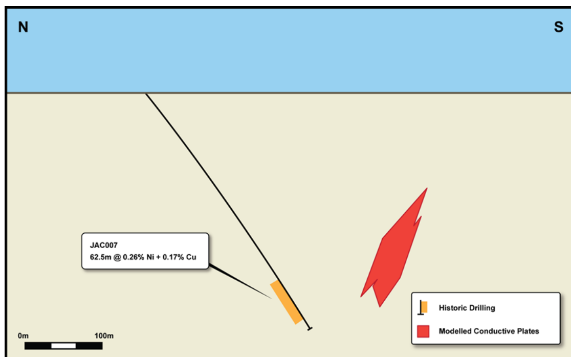
Figure 17: Section looking east through drill hole JAC007 showing the Ni-Cu sulphide intersection and newly detected FLTDEM conductors at the Area 4 prospect.
