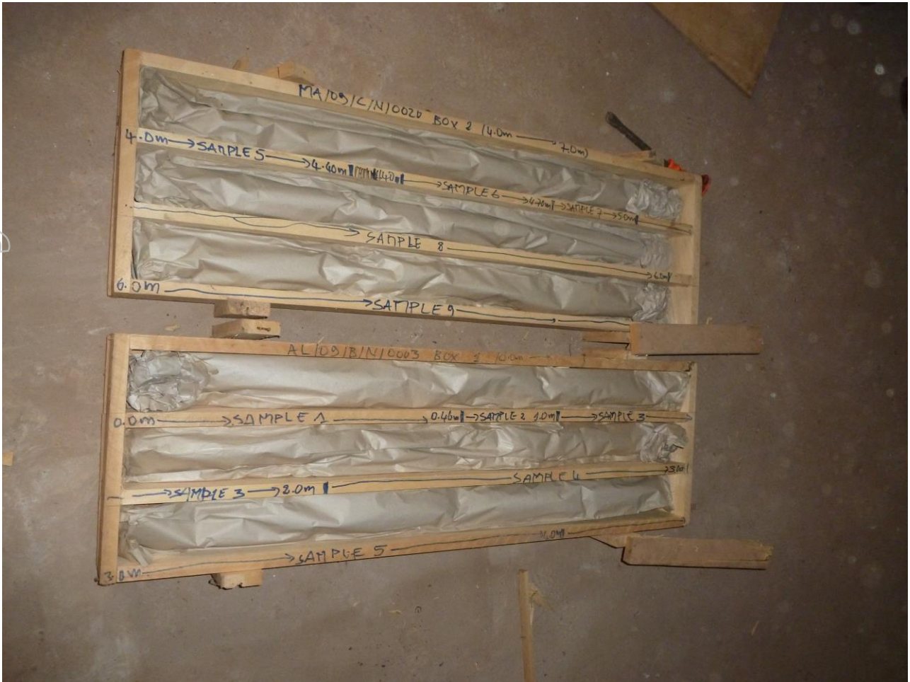
Figure 5: An example of the high quality storage of the drilling core, sealed in wooden boxes and covered
