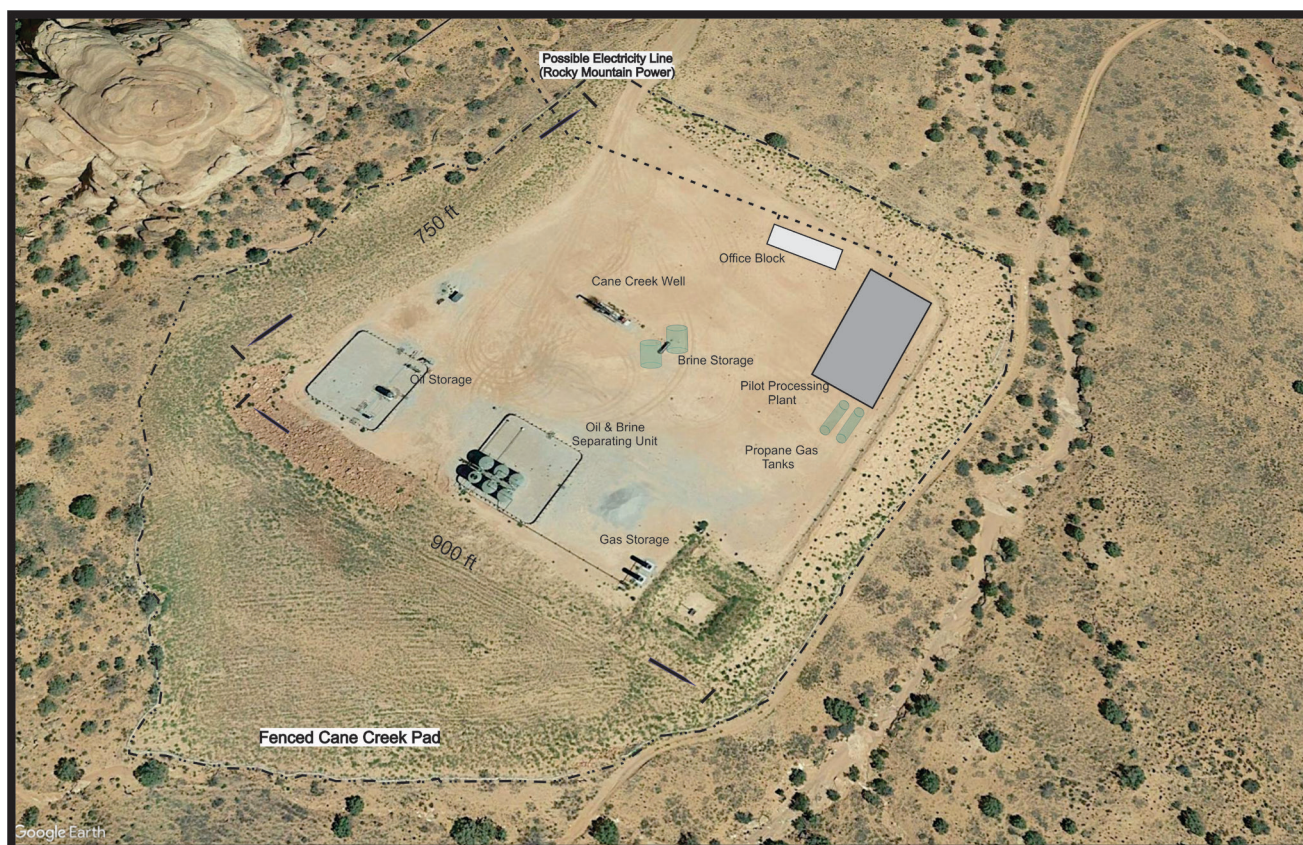
Figure 1: Map showing the proposed location of the pilot plant on the Cane Creek 32-1 Well Pad.
