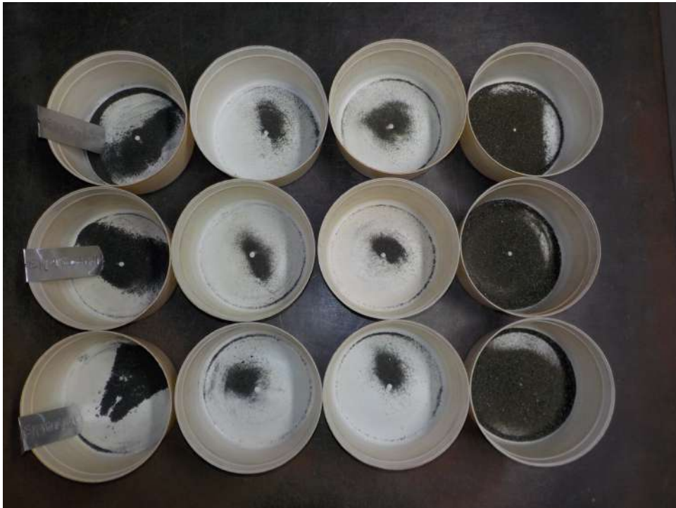
Plate 3 – Magnetic to non-magnetic (left to right) heavy minerals from WHIMS processing The magnetic and the non-magnetic heavy minerals will be subjected to additional analysis to determine if any additional processing stages can increase the value of the concentrates. The three pilot plant tests and related mineral analyses are expected to be completed during the March quarter. A larger bulk sample will then be processed to create samples of products that will be used to for assessment by potential buyers.
