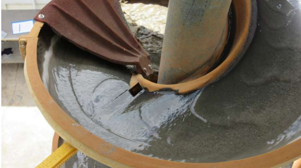
Plate 2 – Spiral separation of heavy minerals (dark grey colour toward centre) from lighter sand using a spiral bank
