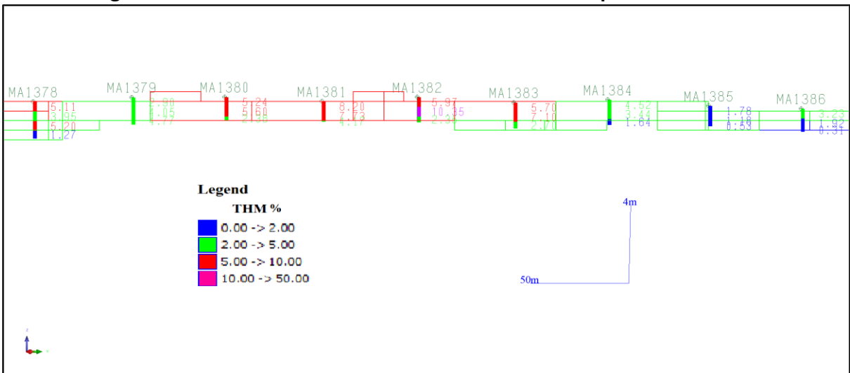
Figure 5 Cross section showing good correlation between block model input drill holes and resource blocks.
