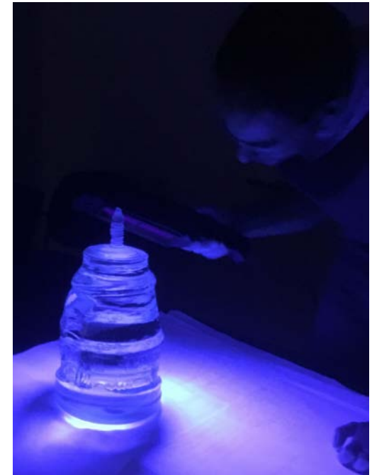
Quality testing of a Polar Sapphire Boule
