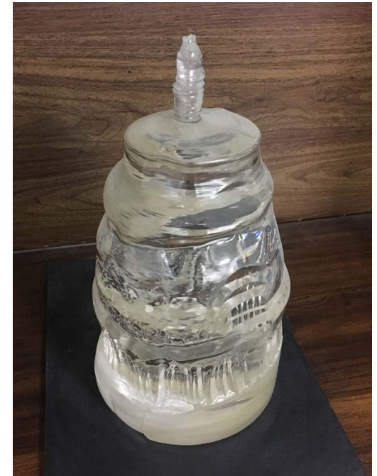
Sapphire Boule made from Polar Sapphire Technology
