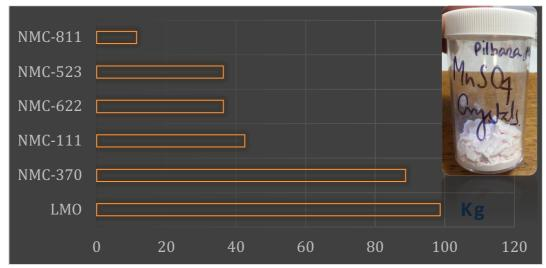
Contained Manganese (per Kg) in a 90Kw/H Battery Pack
