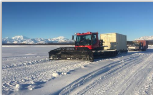
Photo 2-3: Typical snow road freight haul operations in same area as Estelle Gold Project route. Winter road operations bring significant saving from freight costs and allow resource development work to continue unabated year round. Work on road maintenance and freight continues 24/7 during winter months until the job is complete.
