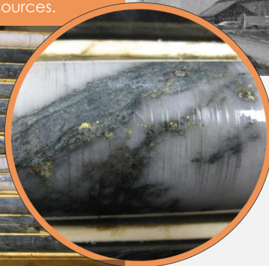
Visible Gold - Pickle Crow Historical High-Grade Diamond Drill Core
