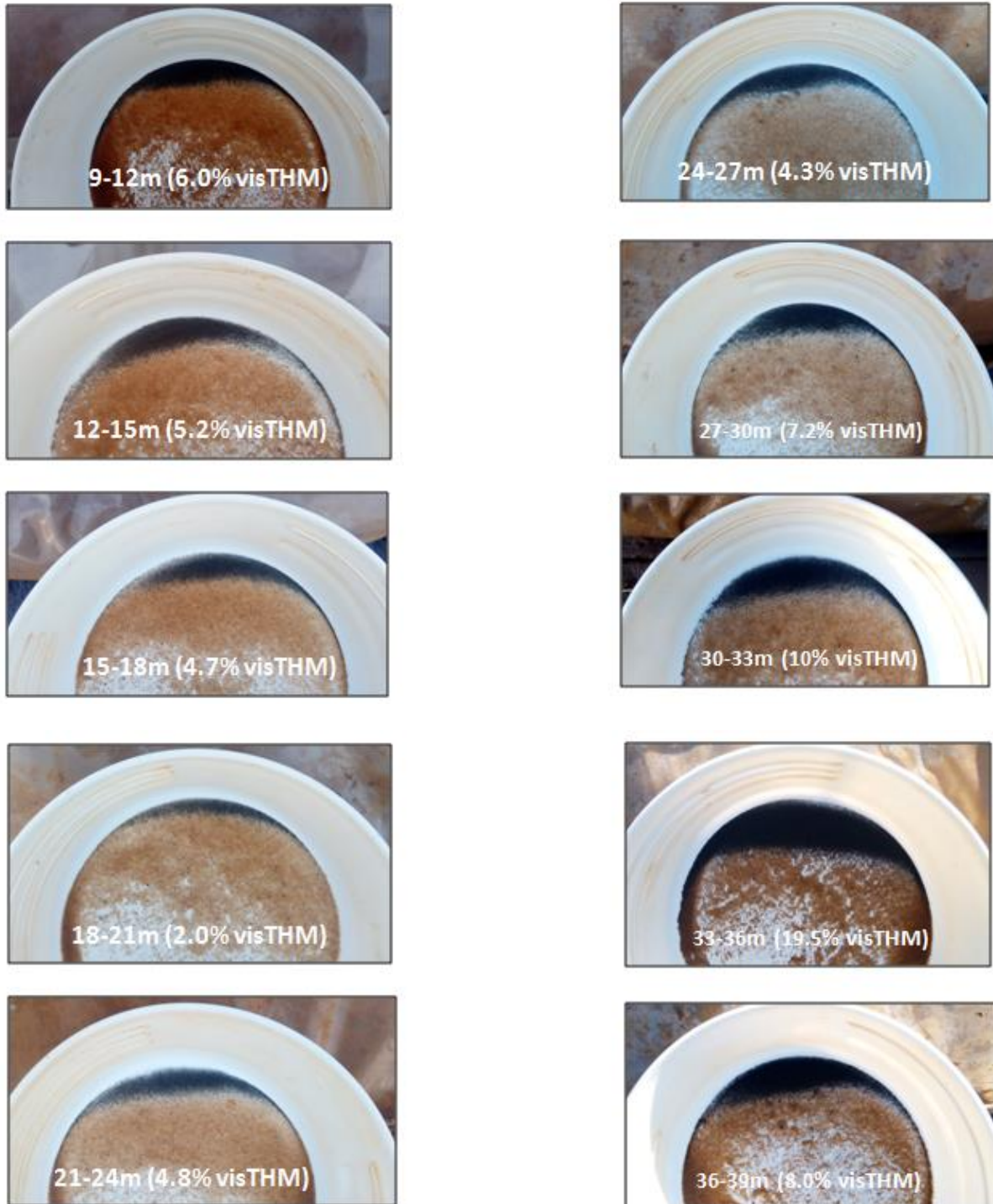
Figure 2: Field pan concentrate photos of samples from Aircore drillhole 20CSAC356 showing an example of a mineralised profile (beginning top left) and the extremely high grades related to strandline style mineralisation (33-36m).
