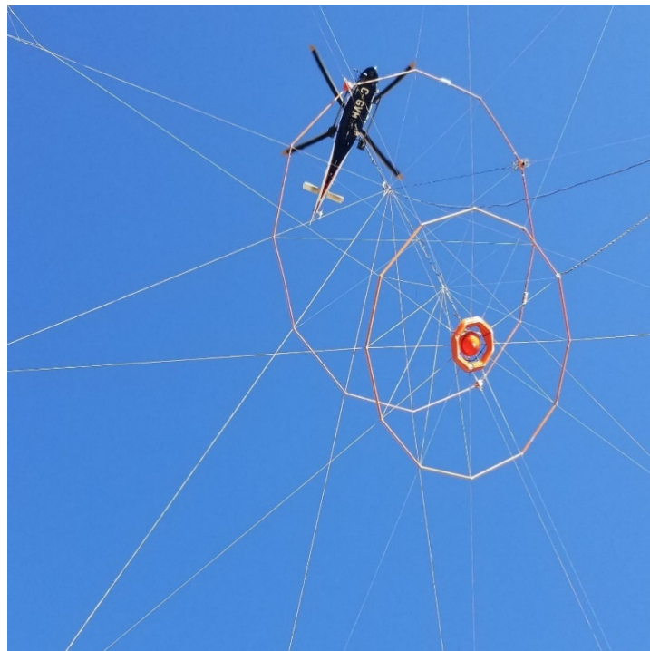
VTEM Plus™ Survey being undertaken at Oracle Ridge
