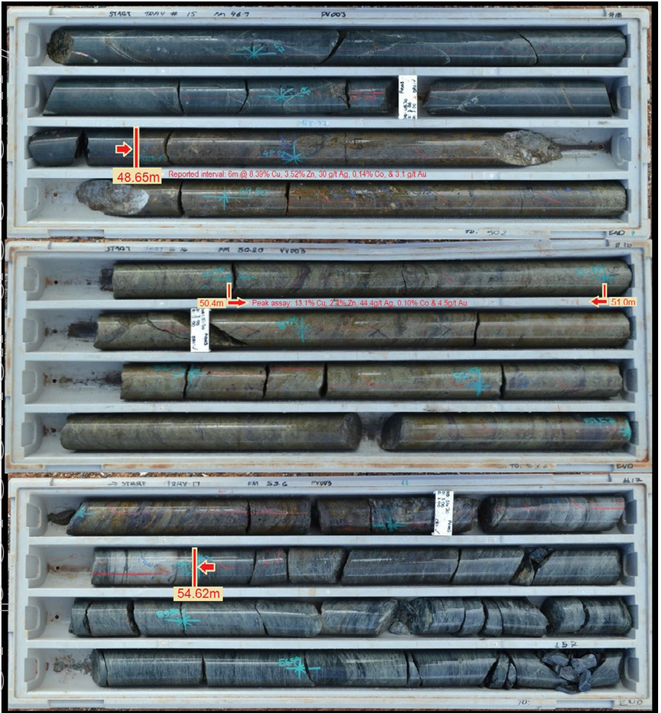
Figure 1: Core trays 15–17 from Schwabe diamond drill hole 20PVDD003 containing primary VHMS mineralisation from 48.65 m to 54.62 m
