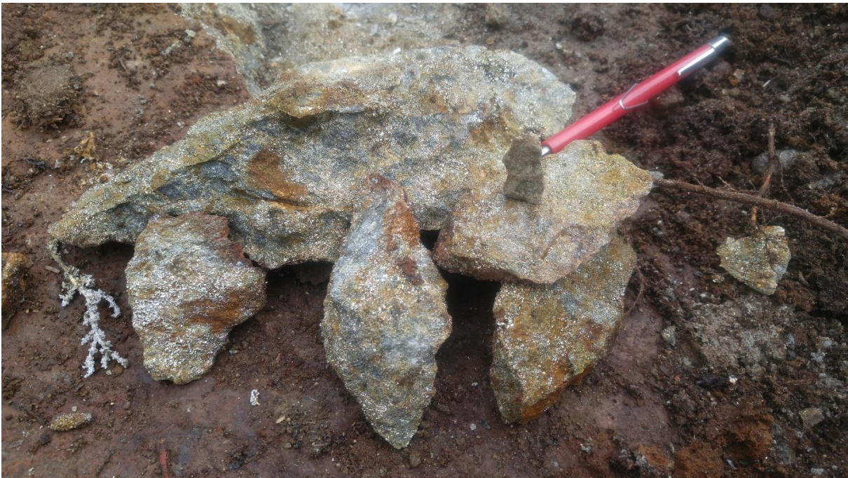
Image 2: Highly silicified, brecciated semi-massive sulphides composed of pyrite, pyrrhotite and minor chalcopyrite (sample #66034), West Carheil Graphitic Trend
