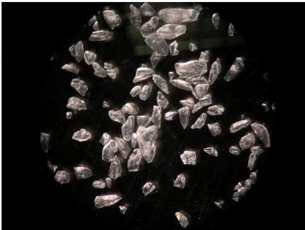
Figure 2: 2 nd Stage lithium hydroxide monohydrate crystallization
