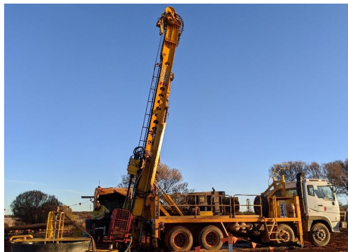
Figure 1: Diamond drill rig on site at the Schwabe Prospect at Perrinvale
