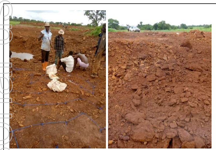
Blast hole charging (LHS) and post-blast laterite iron ore (top left RHS, orange-brown colour) and higher-grade oolitic iron ore, ~52-55% Fe (bottom RHS, dark brown)
