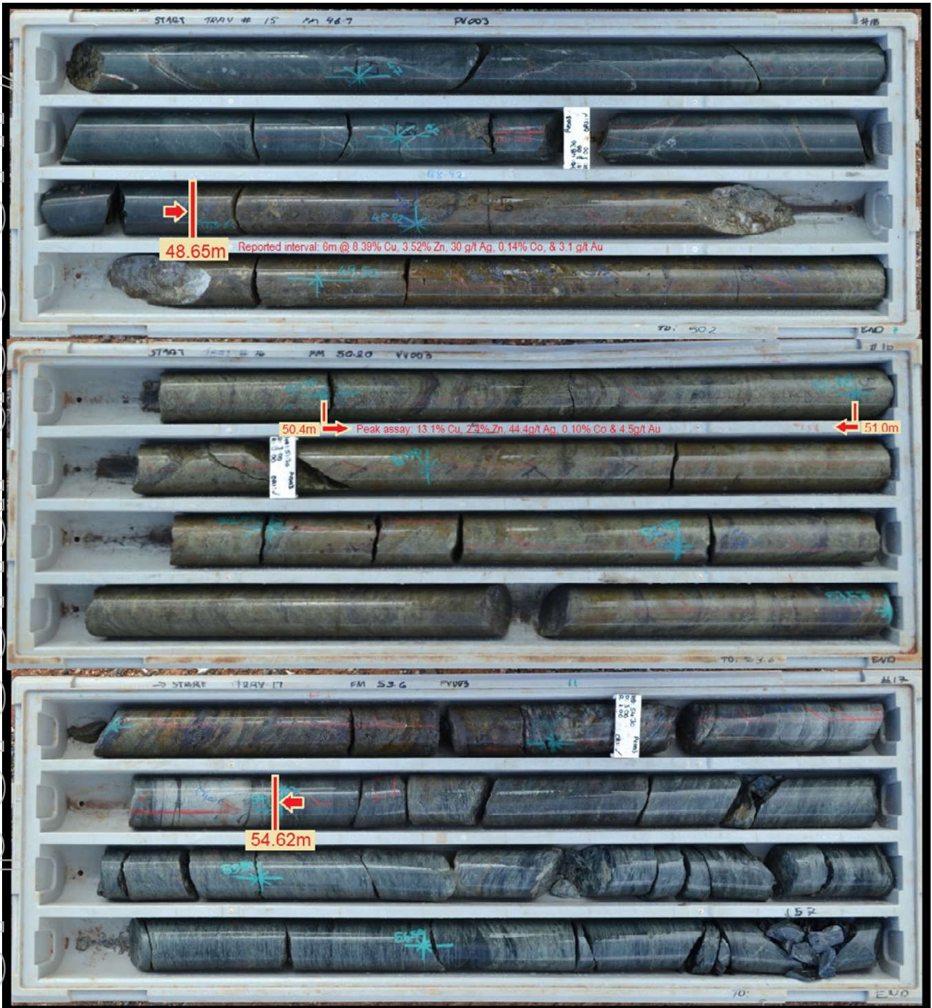
Figure 2: Core trays 15–17 from Schwabe drill hole 20PVDD003 containing primary VHMS from 48.65m to 54.62m
