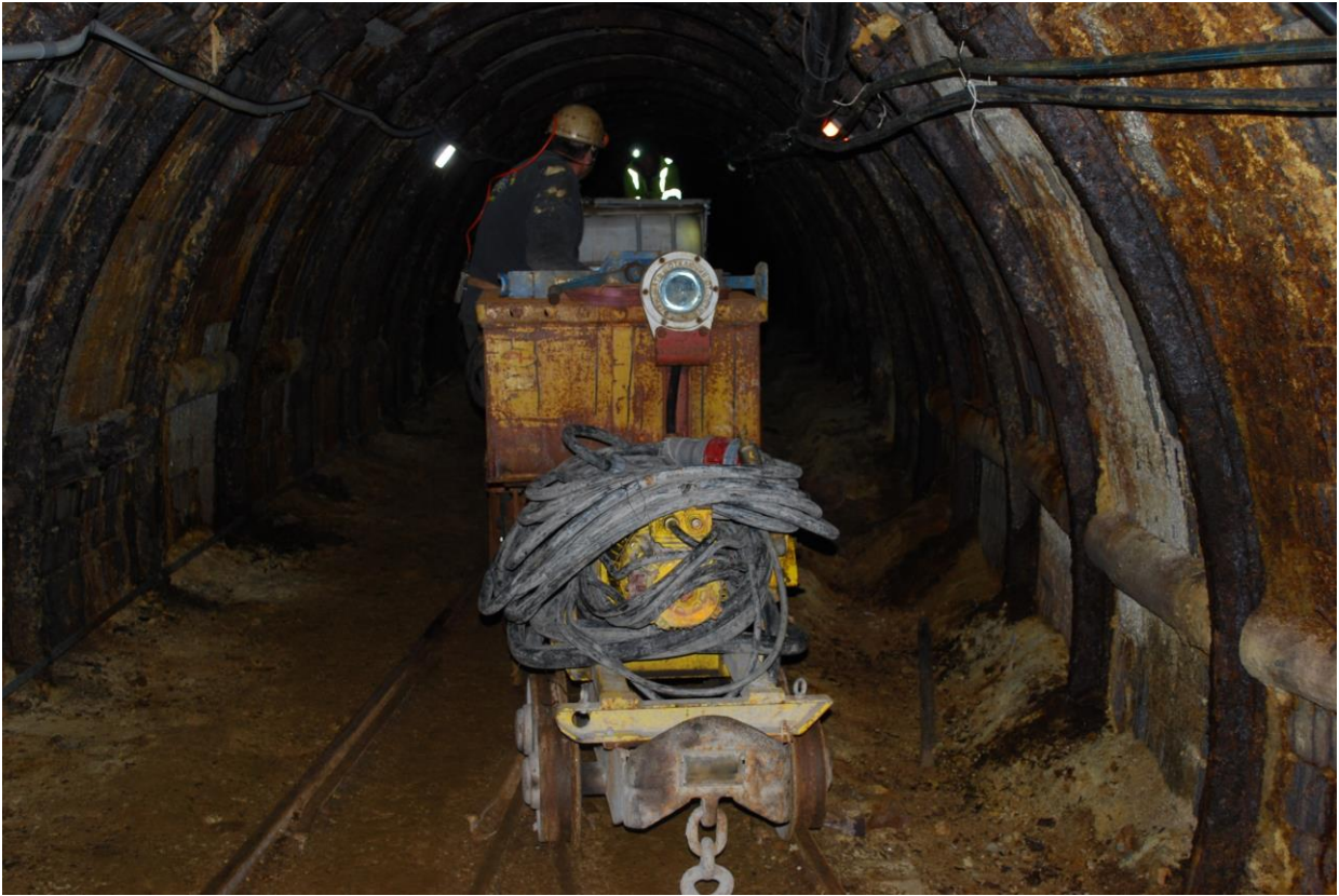
Image 2: Drill rig and ancillary equipment being mobilised to the underground Andrej adit
