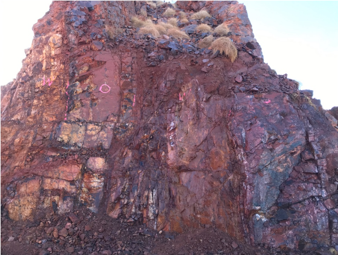
Figure 2. High grade hematite iron ore bands extending from top of ridge to depth
