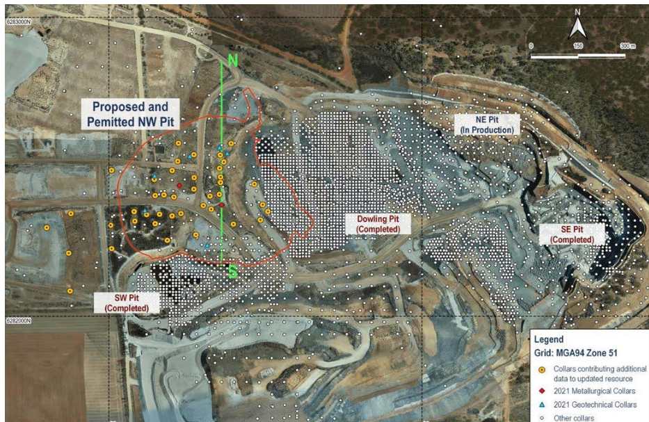
Figure 2: Location map of all additional drilling in the 2NW area since the 2018 Mineral Resource Estimation
