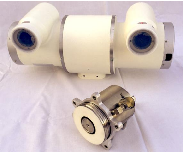
Figure 4: XinRay X-ray source versus a conventional thermionic emitting X-ray tube. The XinRay unit weighs approx 1kg
