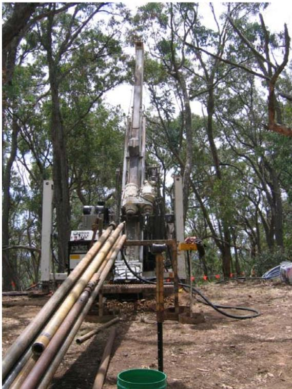
The 2,000m drilling program commenced at Malmsbury on 3 December and a total of 328 metres of drilling was completed by the end of December using a Longyear LF90 diamond drill rig contracted from Silver City Drilling. Logging of the holes is in progress however visual examination as drilling progressed indicated that a number of broken and stock-worked zones have been intersected in this hole.
