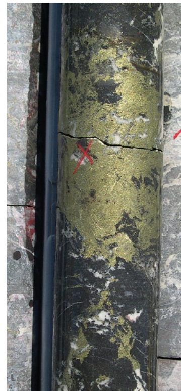
Photo of copper mineralised drillcore from hole R4ARD21, Rover 4 Prospect.
