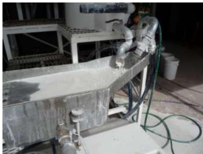
Figure 3: Raw kaolin product prior to filtration
