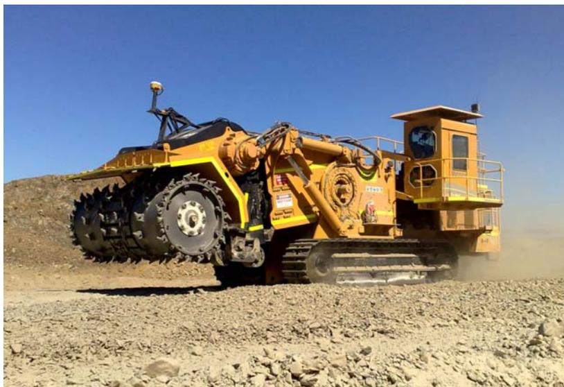
**Figure 4: Resource Test Pit surface continuous miner**
