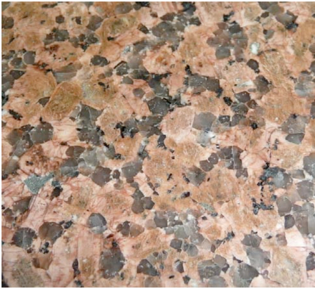
Figure 2: Unweathered granite, surface polished; showing coarse quartz grains, minor mica and feldspar crystals intact
