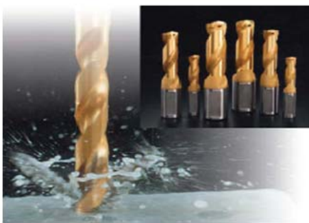
Cemented carbide coated drills improve productivity (Mitsubishi Materials Cooperation & Hitachi Tool Engineering Ltd).
