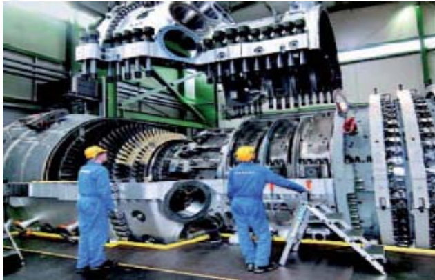
Turbine blades contain up to 10% tungsten. (Siemens AG, Germany).
