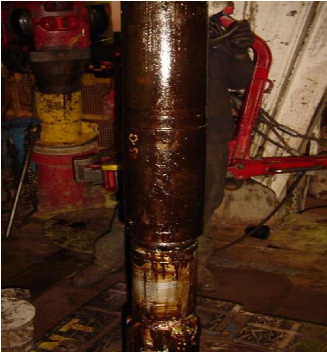
Oil coating 6" bottom hole assembly during horizontal drilling operations at Surprise-1 Re-entry
