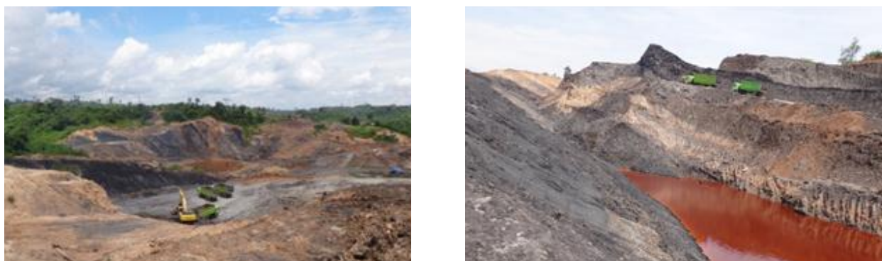
Figure 2: Photographs showing overburden removal at Pit B and haulage from Pit C at Damanka
