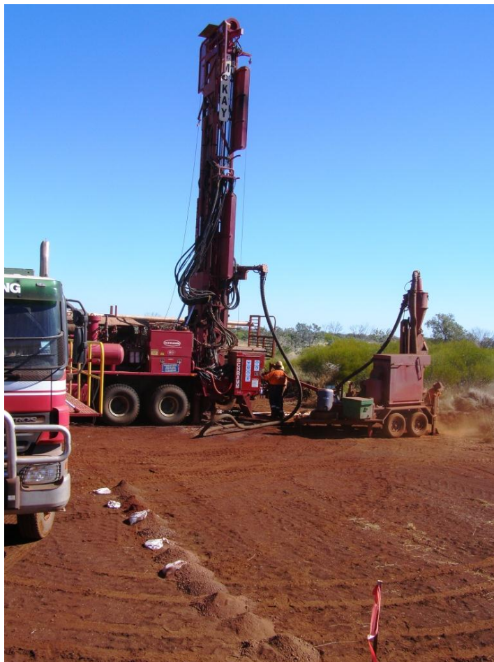
Pic 1: RC drilling at Hamersley Iron Project, June 2012.
