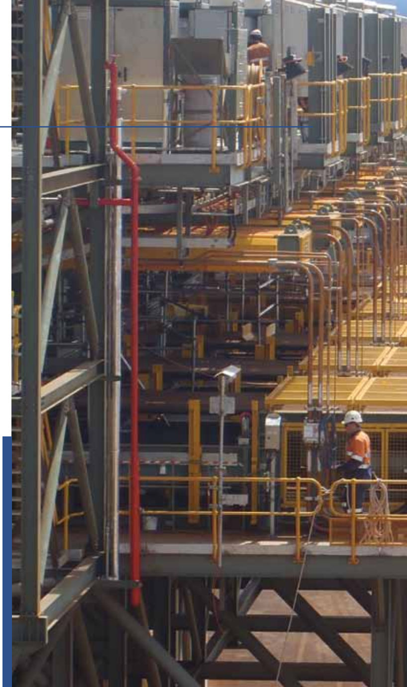
RCR designed, manufactured and supplied 15 belt feeders and 2 large apron feeders, 30 metres long and weighing 220 tonnes for BHPB's operation at Yandi, Western Australia
