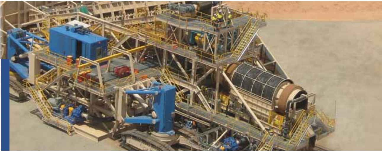
RCR designed - and - built Award winning Mobile In-Pit Crushing and Conveying Unit (IP2C)
