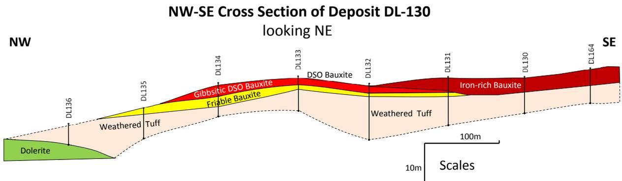
Figure 5: Cross Section Of The Northwest Part of Bauxite Deposit DL-130
