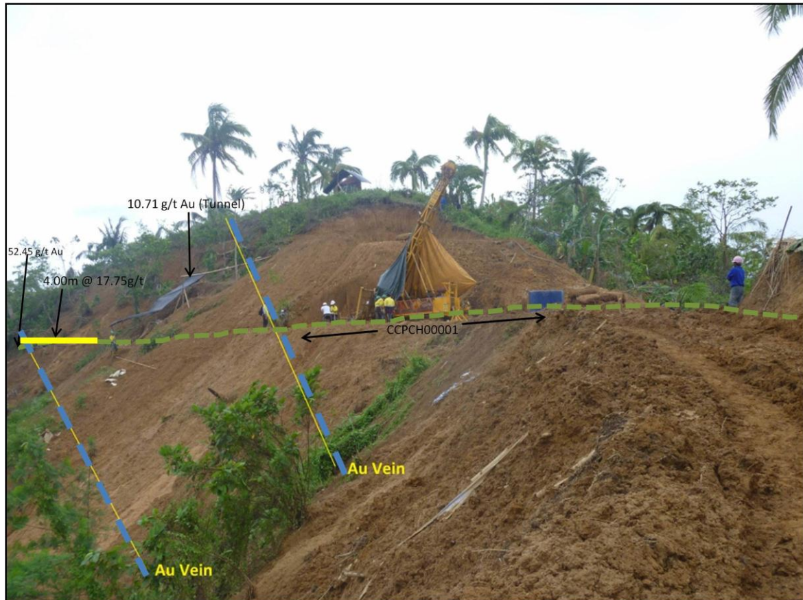
Figure 3 - Drill site for TGPDH00001 showing approximate location of mineralised quartz veins and mineralisation within CCPCH00001
