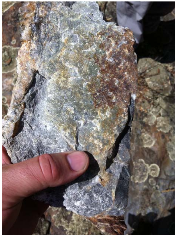
Figure 2: Silica altered, felsic intrusive grab sample taken from discovery outcrop at Numao Project. Visible sulphides along vein edges observed by Plymouth geologist in September 2013.
