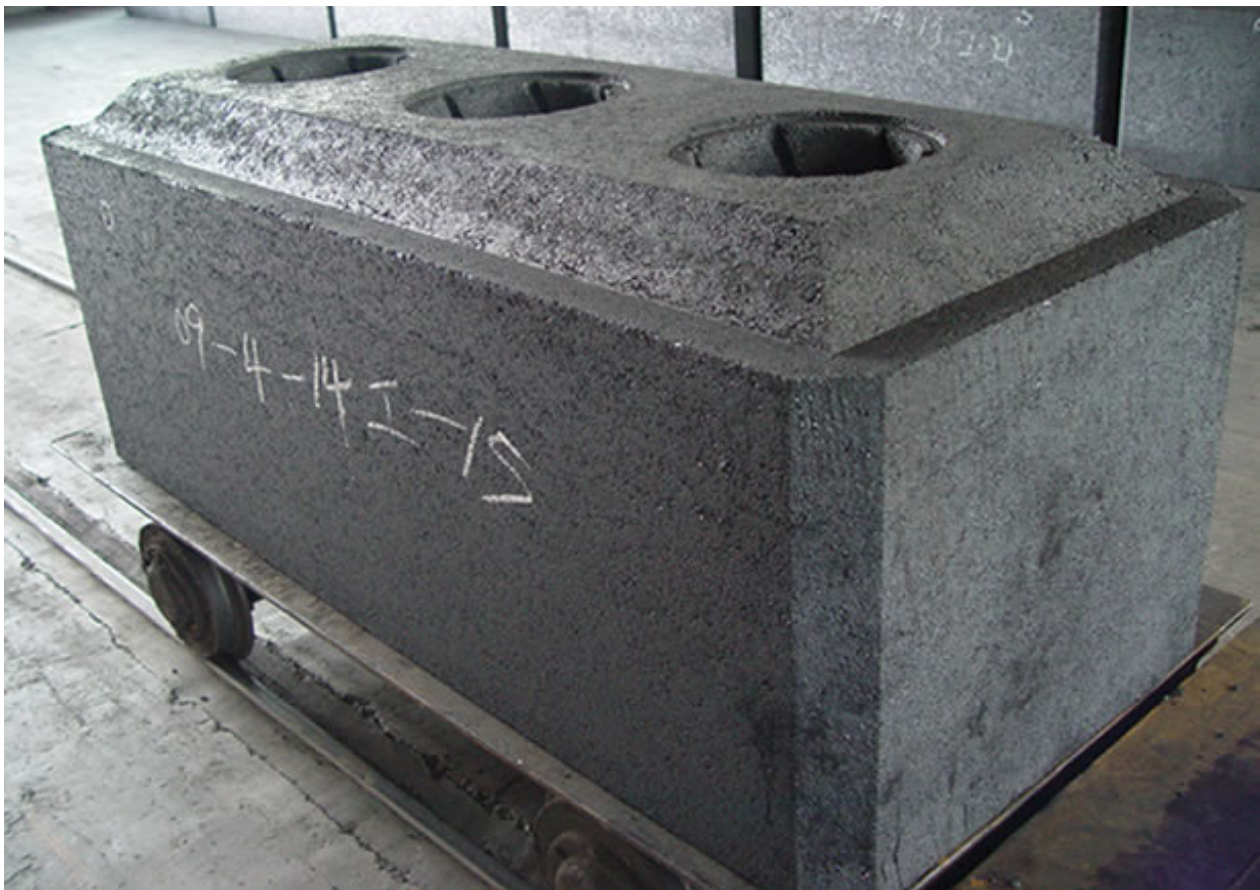
Figure 3 – An anode block used in aluminium smelting (Picture source: Baotou Aluminum (Group) Co. Ltd - member of the Chinalco group ( http://en.baotou-al.com/ ))
