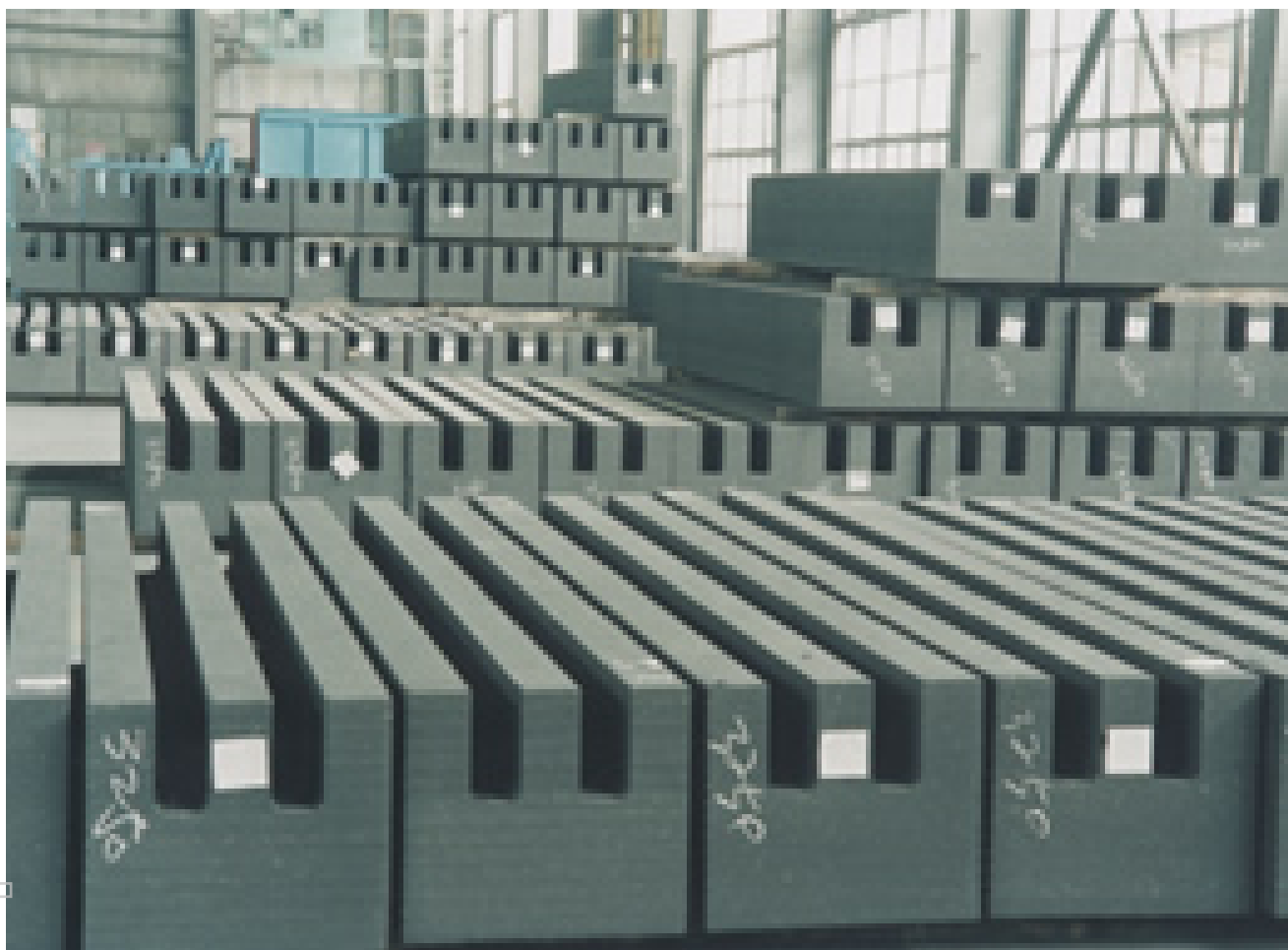
Figure 4 – Cathode blocks used in aluminium smelting. (Picture source: Chinalco ( http://www.chalco.com.cn ))
