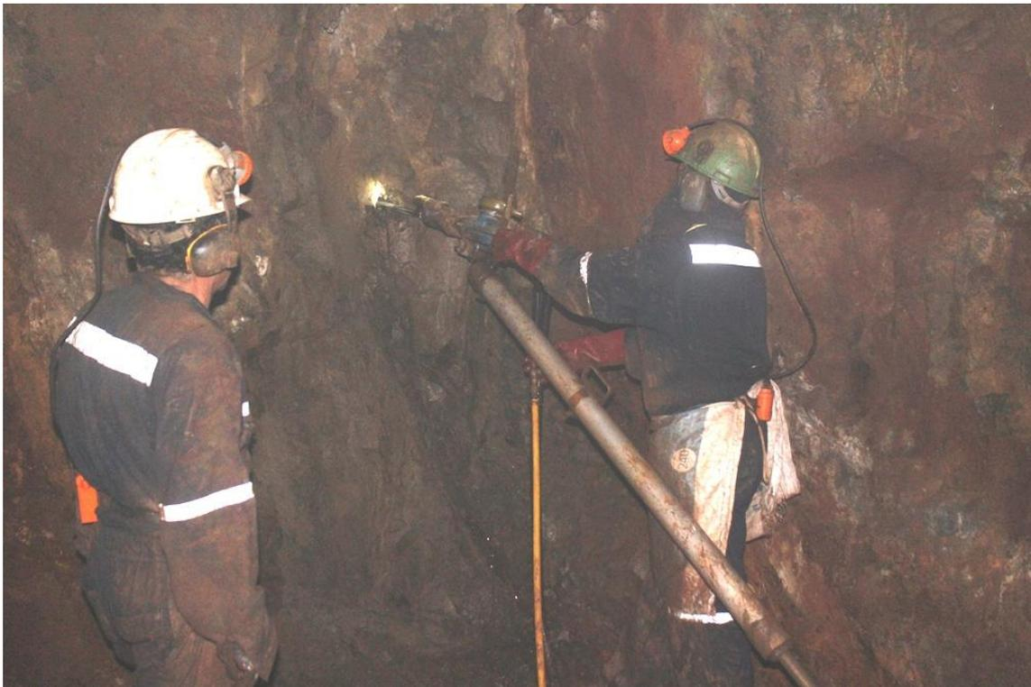
**Figure 3 – Underground airleg miners on the 966 Level at Panga Mine.**
