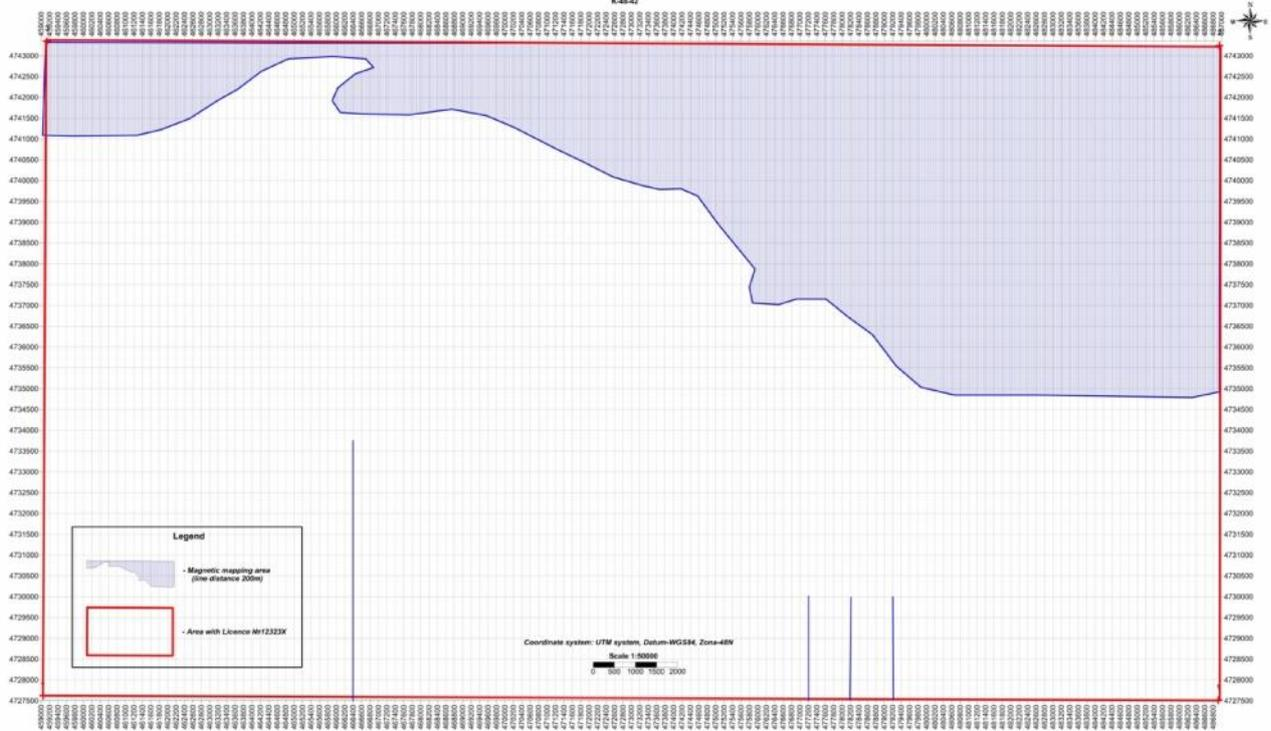
**Figure 3:** Newera Resources Ltd Ulaan Tolgoi project licence plan, inclusive of an outline of the May 2014 ground magnetics survey plan on 200 metre line spacing for a total of ~ 700 line kilometers of ground magnetics surveying. See Appendix A for clarity.
