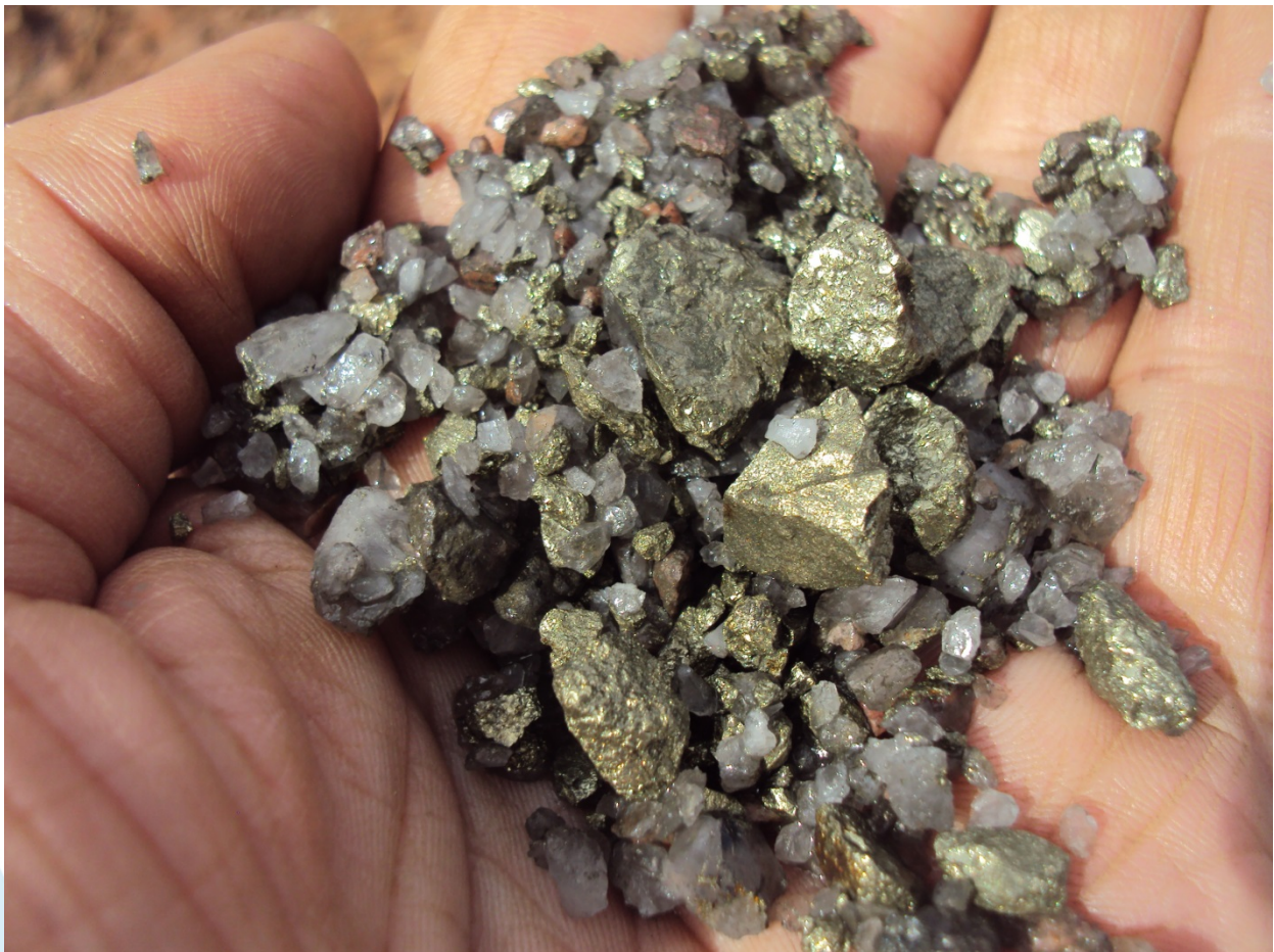
Figure 2: RC chips from hole BYRC018 – the brassy yellow mineral in abundance is the copper sulphide, chalcopyrite
