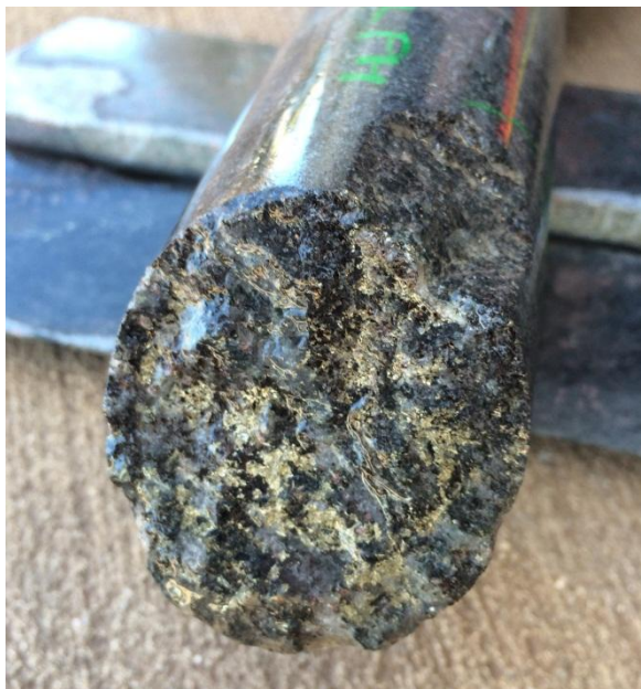
Figure 1. Disseminated sulphides in core
