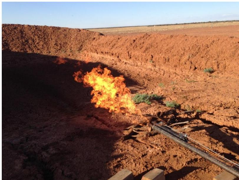
Figure 1 – Flare from flow test at Queenscliff-1
