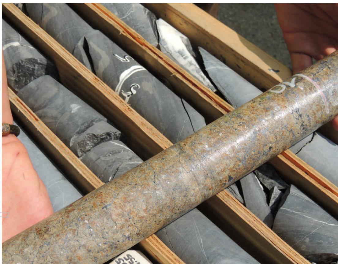
Figure 1 Massive zinc sulphides with brown sphalerite and grey galena in GDD004
